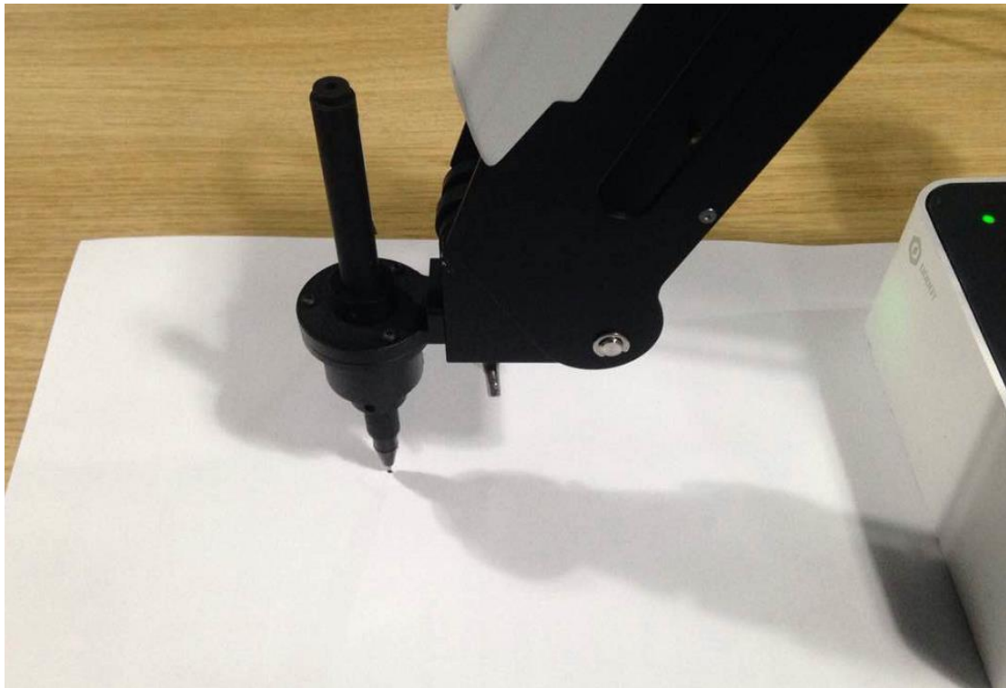
Figure 4.12 Adjust the nib position
