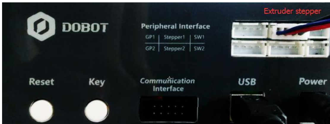
Figure 7.5 Connection of extruder
