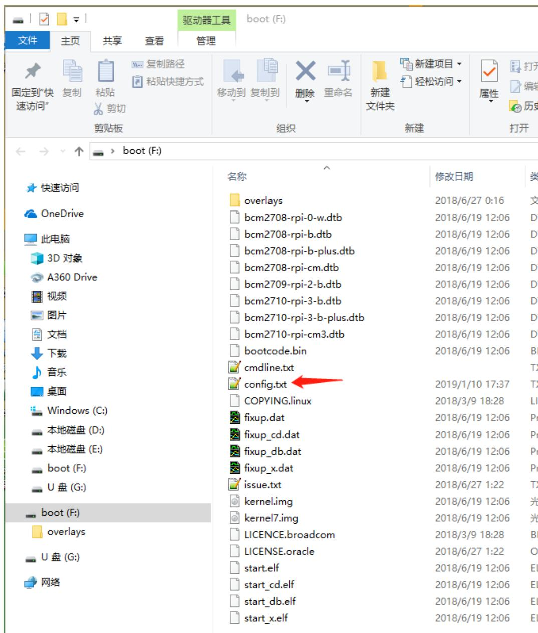
Open the Raspberry Pi startup TF card on the computer and find the config.txt startup configuration file.
